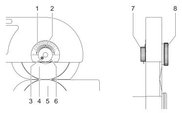
Fig. 5 Adjustment of the stop of the upper blade
