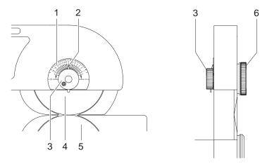
Fig. 4 Height adjustment of the upper blade
