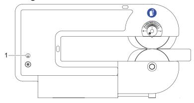
Fig. 3 Earthing Connection
