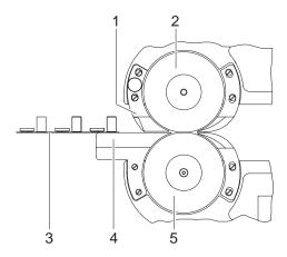
Fig. 7 Separation of the PCB's
