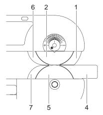
Fig. 8 Alignment of blades and guides
